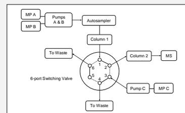
Figure 1. Valve-switching setup for on-line cleanup
